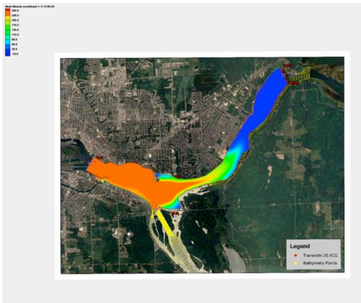
Fig. C5. Simulation of sediment transport in St. Marys River under low flow condition: Elapsed time = 12.0 hrs.
