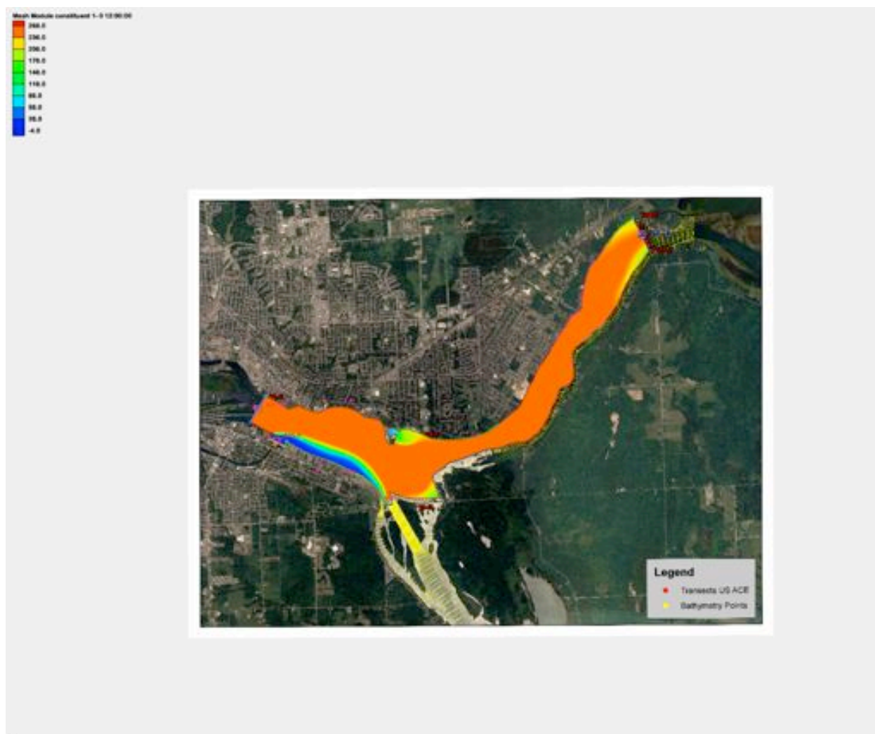
Fig. C10. Simulation of sediment transport in St. Marys River under high flow condition: Elapsed time = 12.0 hrs.
