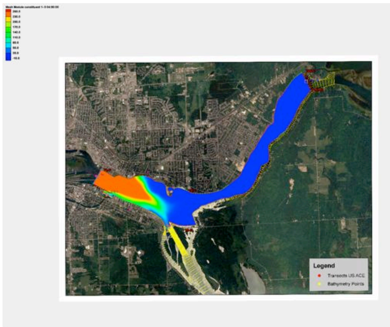
Fig. C3. Simulation of sediment transport in St. Marys River under low flow condition: Elapsed time = 4.0 hrs.
