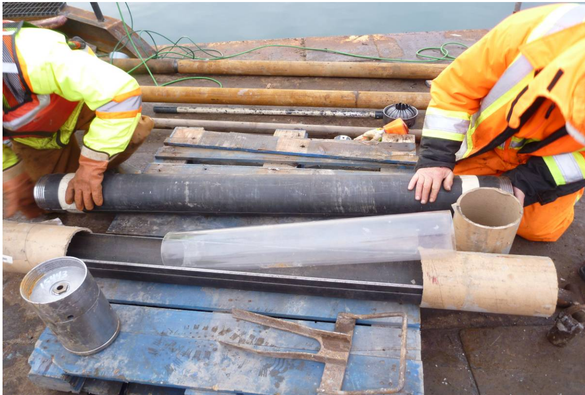
Photograph #7 – 130 mm inside \varnothing split-barrel sampler with acrylic sleeves, and sampling head
