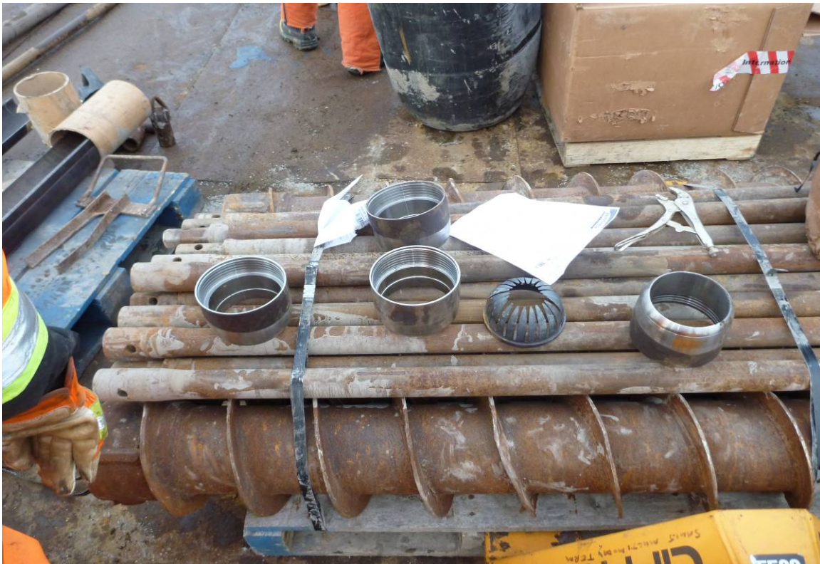
Photograph #6 – 250 mm ø hollow stem augers and 51 mm ø drill rods
