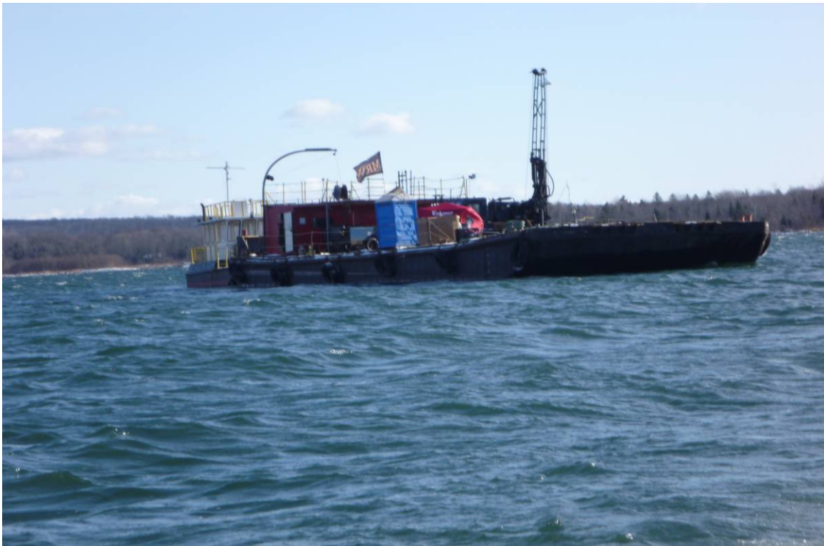
Photograph #1 – 100 tonne capacity barge with drill rig mounted on it
