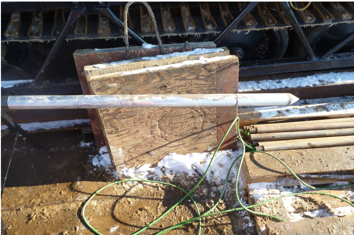
Photograph #8 – Electronic piezocone c/w Ultra Violet Induced Fluorescence (UVIF) module
