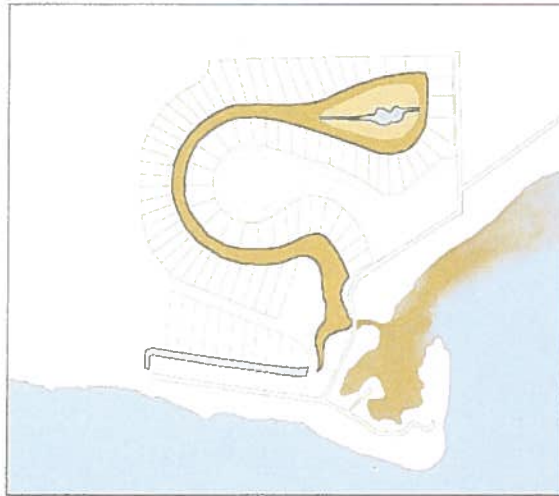
Conceptual Model of Canal Water Migration Along the Shoreline of the St. Marys River from the Inlet Bay
