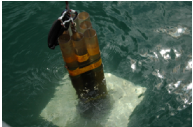
Photograph on the left depicts the positioning of the in situ flume for sediment stability experiments. Photograph on the right depicts the recovering of the bottom mounted sediment traps for sediment stability experiments. Photo credits: Johann (Hans) Biberhofer, Environment Canada.
