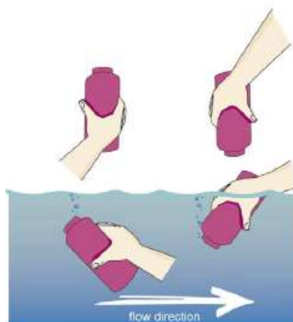
Figure 2: Grab-sampling method (source: CCME 2011)
