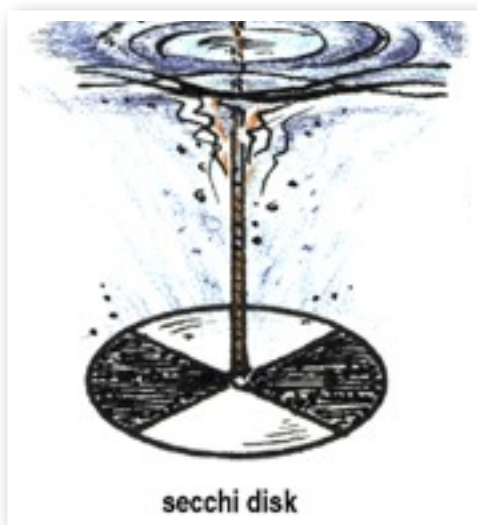
The Secchi disk is a device used to measure water clarity.
